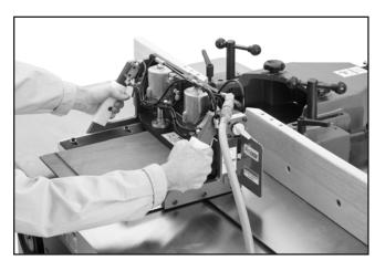
Figure 20. Shaping jig in use.
